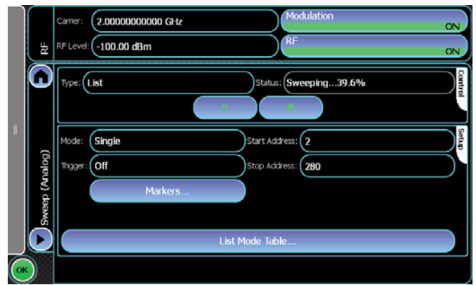
List Mode control screen showing a List sweep in action
